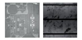
At wavelengths above 1100 nm silicon becomes transparent. Thus, SWIR cameras are perfect for analyzing metallization and electrical contact errors on the backside of wafers.
