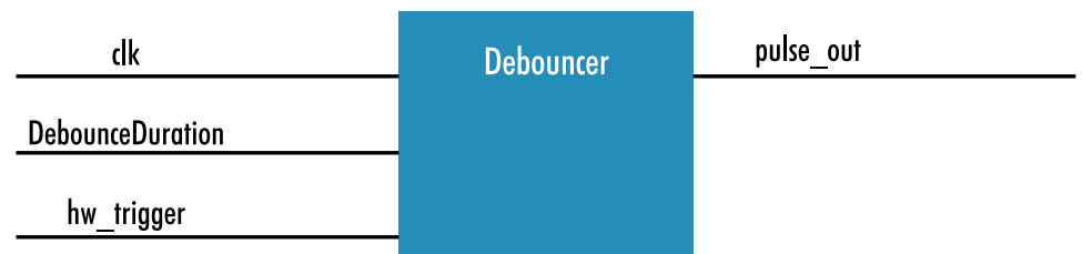
Fig. 5-52: The debouncer module
