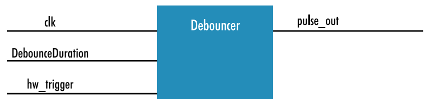
Fig. 5-44: The debouncer module
