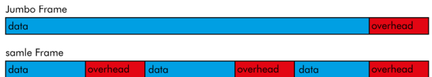
Fig. 3-2: Data reduction with jumbo frames
