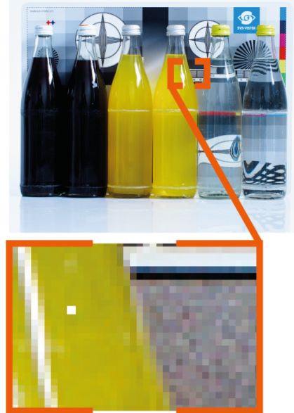
Fig. 5-23: Illustration of a defect pixel
