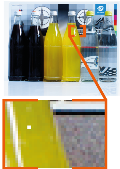
Fig. 5-26: Illustration of a defect pixel
