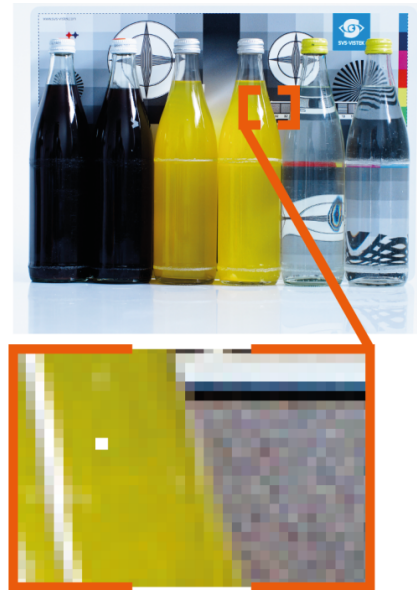
Fig. 5-22: Illustration of a defect pixel
