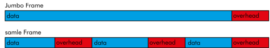
Fig. 3-3: Data reduction with jumbo frames
