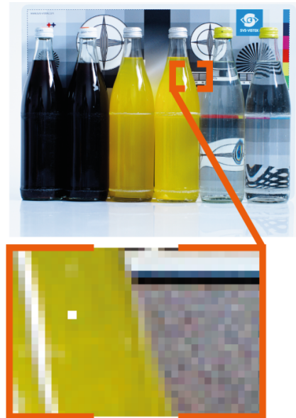
Fig. 5-22: Illustration of a defect pixel
