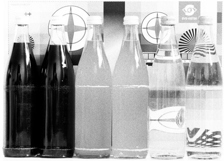
Fig. 5-1: Noise caused by too much gain
