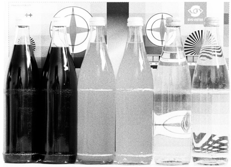
Fig. 5-1: Noise caused by too much gain
