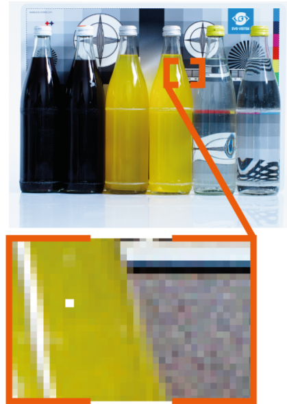
Fig. 5-27: Illustration of a defect pixel
