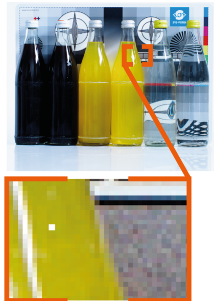
Fig. 5-27: Illustration of a defect pixel
