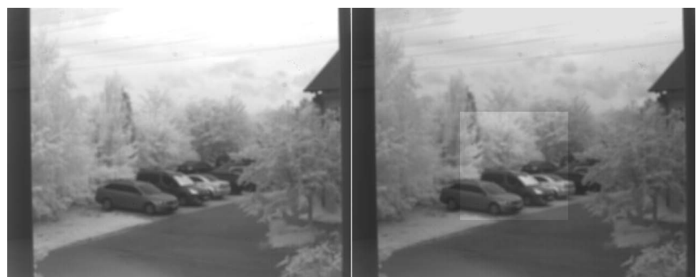
Figure 96: Example for the effect of AutoModeRegionDimOutside. Left: without dimming applied, right: with dimming applied to the outside area.
