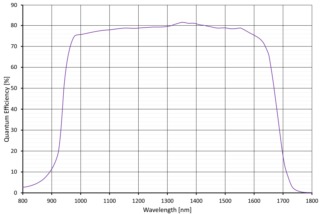
Figure 17: Goldeye CL-008 SWIR TEC1 absolute QE
