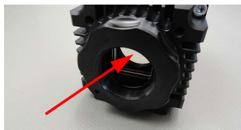
Figure 108: Camera mount without filter, directly exposing the sensor
