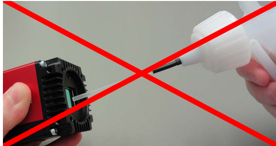
Figure 111: How not to use compressed air
