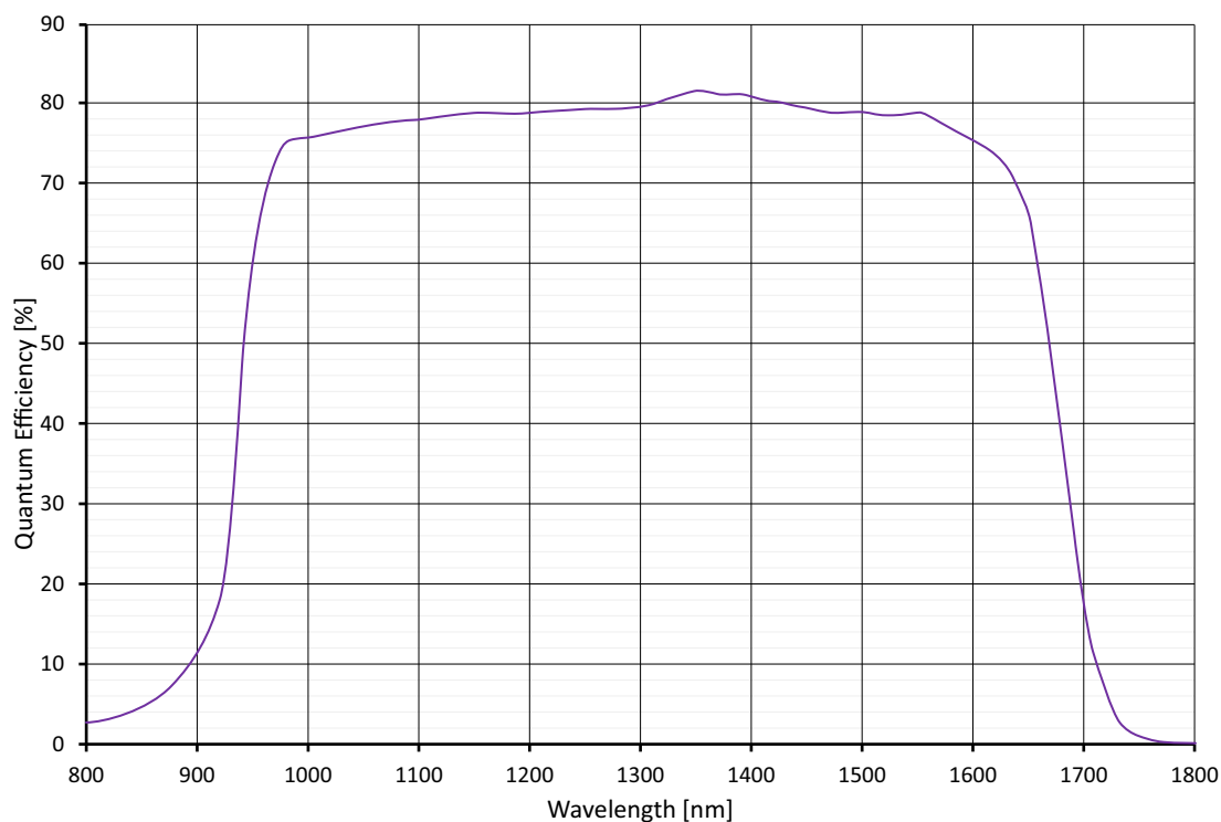
Figure 18: Goldeye CL-008 SWIR Cool TEC1 absolute QE
