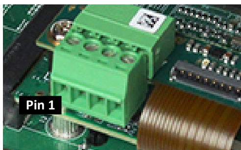
Figure 7: Adapter for Wandboard i.MX6 | I/O terminal, wiring diagram
