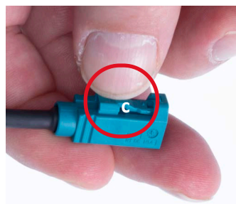
Figure 10: Pressing down the latch (c) of the FAKRA coaxial connector
