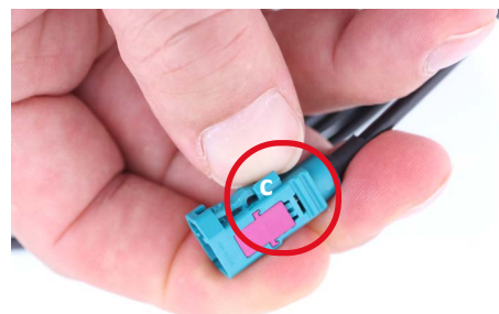
Figure 11: Pressing down the latch (c) of the HSD STP connector
