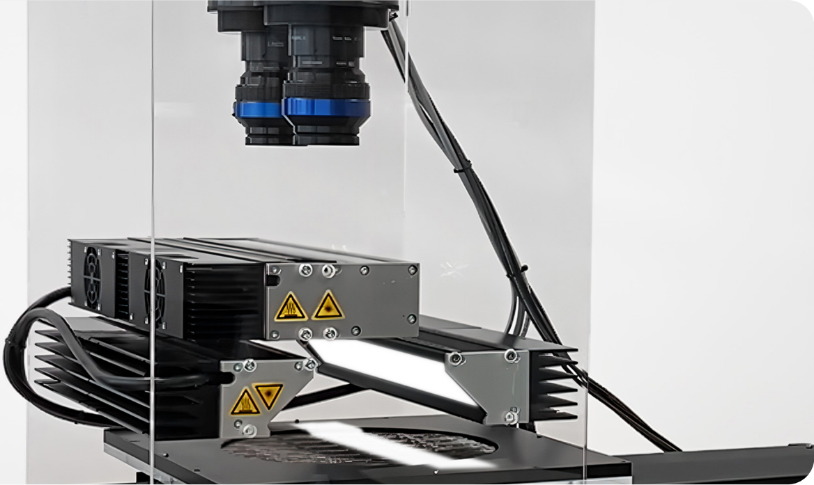
Wafer scanner set-up with two allPIXA evo 16k line scan cameras and combined light: Corona II dark field and coaxial light
