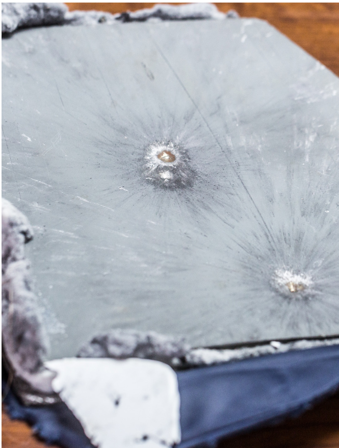
Bulletproof armored plates passed the test after being fired upon with firearms.
