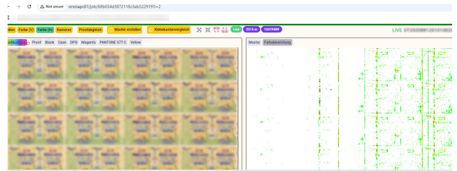
VInspect interface: Display of color deviation in the current print image (right) in relation to the reference (left). White: no color deviation. Green: slight color deviation.
